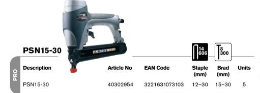
Ideal for cabinet-making, mouldings, etc. Can be used with narrow crown staples or brads. Switch-controlled changeover from single shot action to automatic firing action. Protective pad to avoid scratching surface.
