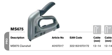
Combi cable tacker for low-voltage cables. Rapid 7: max diameter 6.0 mm. Rapid 17: max diameter 7.5 mm.
